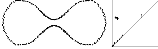
Figure 4: A point cloud \mathbb{X} (left) and the zero-dimensional persistence diagram (right). The values r and s are half the distance between the two top clusters and between the right and bottom cluster, respectively.
